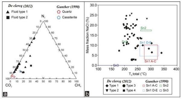
**Fig:8:** (a)  $CO_2$ -N<sub>2</sub>-CH<sub>4</sub> Ternary diagram showing the composition of the gas phase of luid inclusions from quartz and cassiterite crystals in Sn mineralised veins from the Rutongo area by Günther (1991) and De clercq (2012). (b) Scatter plot of T<sub>h,tot</sub> versus Salinity of fluids from Sn-mineralised quartz veins from the Rutongo area in Rwanda, by Günther (1991) and De clercq (2012).
